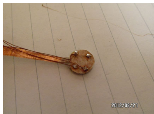
Figure 19: Solder copper leads.
