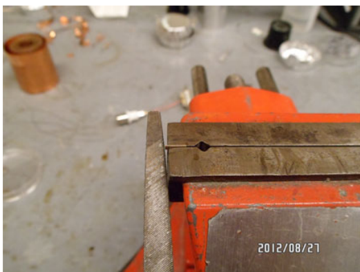
Figure 11: Plane the foil.
