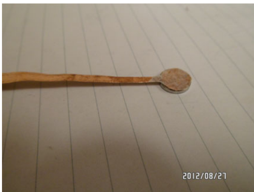
Figure 16: Varnish the copper foil onto the bottom spacer.
