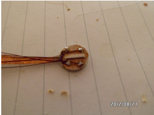
Figure 20: Varnish the manganin foil.
