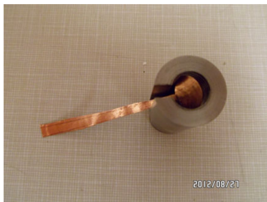
Figure 14: Test the copper foil in the pressure cell.
