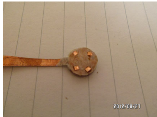
Figure 18: Varnish four small pieces of copper foil.
