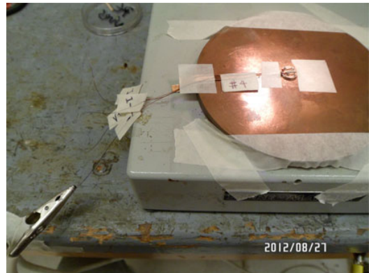
Figure 22: Connect Pt wire to the soldering points.
